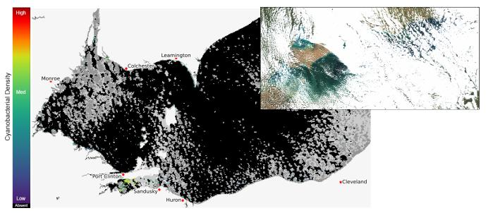
Current Lake Erie Sentinel-3 satellite imagery from the Ocean and Land Color Imager (OLCI) on Oct 22, 2023, showing bloom location and extent in the western basin. Grey indicates clouds or missing data. The estimated threshold of cyanobacteria detection is 20,000 cells/mL. Inset shows a truecolor image of the entire lake. Data derived from Copernicus Sentinel-3.
