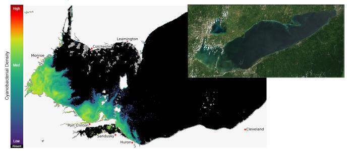
Current Lake Erie Sentinel-3 A and B composited satellite imagery from the Ocean and Land Color Imager (OLCI) on Sep 02, 2021, showing bloom location and extent in the western basin. Grey indicates clouds or missing data. The estimated threshold of cyanobacteria detection is 20,000 cells/mL. Inset shows a truecolor composite image of the entire lake. Data derived from Copernicus Sentinel-3.
