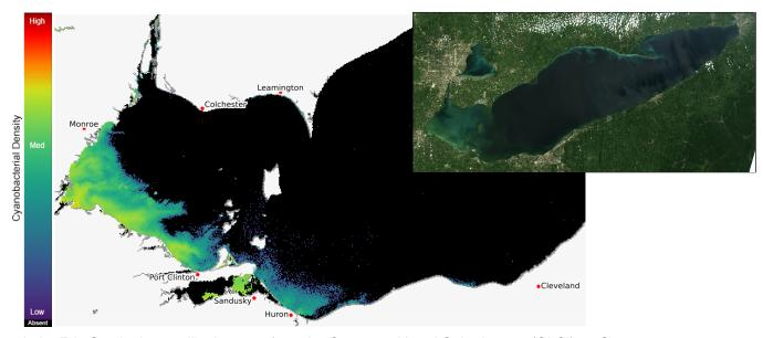
Current Lake Erie Sentinel-3 satellite imagery from the Ocean and Land Color Imager (OLCI) on Sep 01, 2023, showing bloom location and extent in the western basin. Grey indicates clouds or missing data. The estimated threshold of cyanobacteria detection is 20,000 cells/mL. Inset shows a truecolor image of the entire lake. Data derived from Copernicus Sentinel-3.
