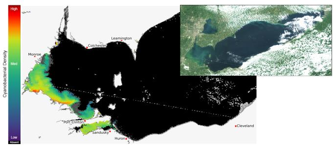
Current Lake Erie Sentinel-3 satellite imagery from the Ocean and Land Color Imager (OLCI) on Aug 04, 2023, showing bloom location and extent in the western basin. Grey indicates clouds or missing data. The estimated threshold of cyanobacteria detection is 20,000 cells/mL. Inset shows a truecolor image of the entire lake. Data derived from Copernicus Sentinel-3.
