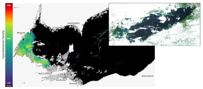
Current Lake Erie Sentinel-3 satellite imagery from the Ocean and Land Color Imager (OLCI) on Aug 26, 2023, showing bloom location and extent in the western basin. Grey indicates clouds or missing data. The estimated threshold of cyanobacteria detection is 20,000 cells/mL. Inset shows a truecolor image of the entire lake. Data derived from Copernicus Sentinel-3.
