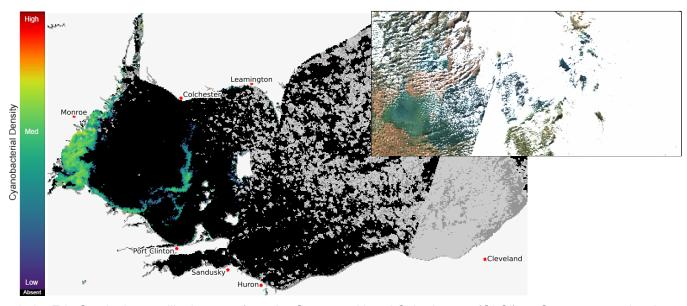
Current Lake Erie Sentinel-3 satellite imagery from the Ocean and Land Color Imager (OLCI) on Oct 13, 2022, showing bloom location and extent in the western basin. Grey indicates clouds or missing data. The estimated threshold of cyanobacteria detection is 20,000 cells/mL. Inset shows a truecolor image of the entire lake. Data derived from Copernicus Sentinel-3.
