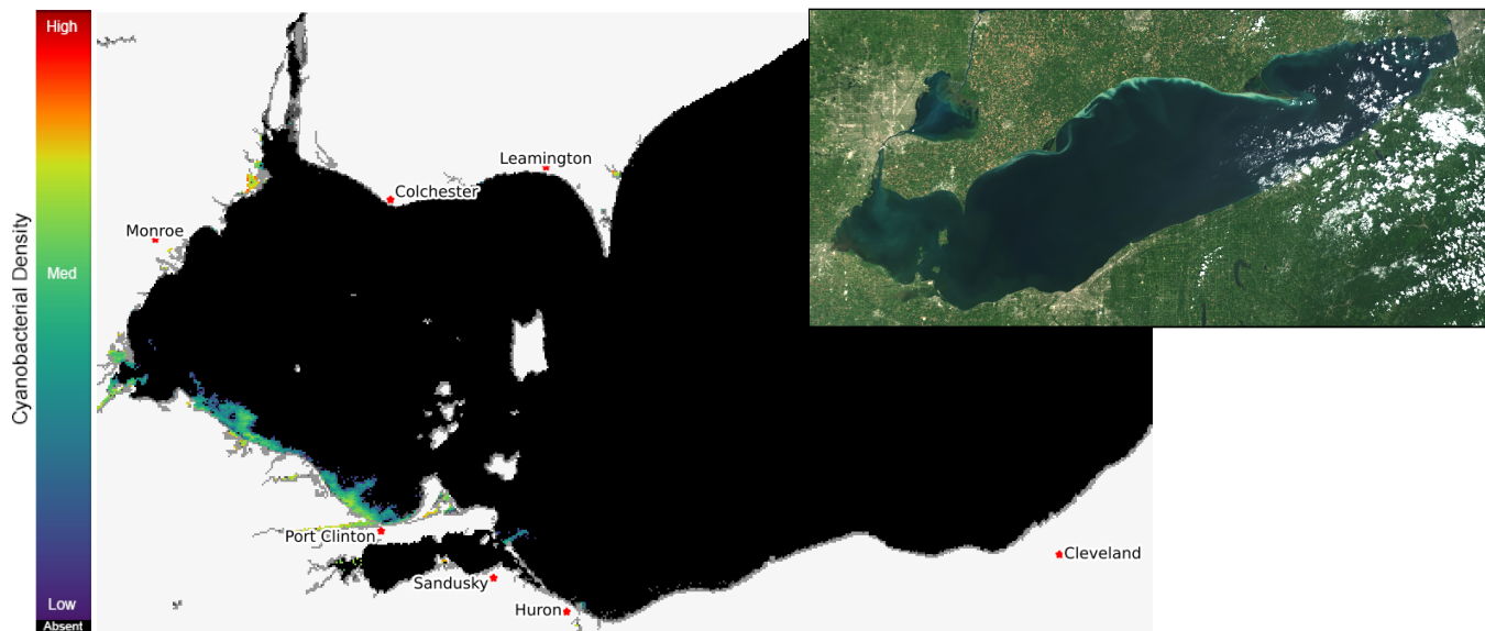
Lake Erie current Sentinel-3B satellite imagery from the Ocean and Land Color Imager (OLCI) on Jul 26, 2021, showing bloom location and extent in the western basin. Grey indicates clouds or missing data. The estimated threshold of cyanobacteria detection is 20,000 cells/mL. Inset shows truecolor image of the entire lake. Data derived from Copernicus Sentinel-3.
