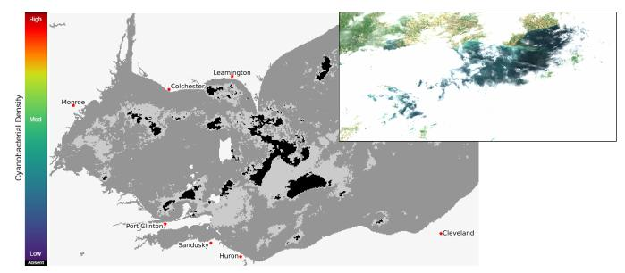
Current Lake Erie Sentinel-3 satellite imagery from the Ocean and Land Color Imager (OLCI) on May 15, 2024, showing bloom location and extent in the western basin. Grey indicates clouds or missing data. The estimated threshold of cyanobacteria detection is 20,000 cells/mL. Inset shows a truecolor image of the entire lake. Data derived from Copernicus Sentinel-3.
