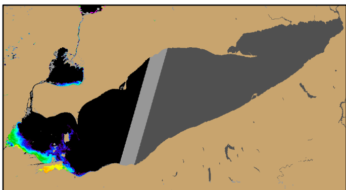
Figure 2. Cyanobacterial Index from modified Copernicus Sentinel 3 data collected 23 August, 2018 at 12:12.
